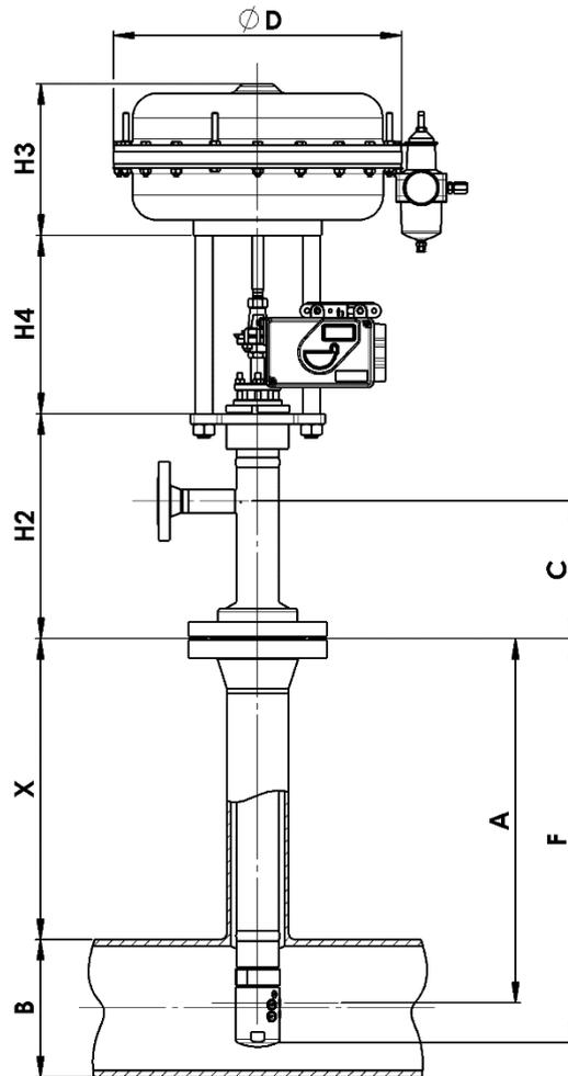
The variable dimension is X, in order to have the Sprayhead in the center of the pipe
